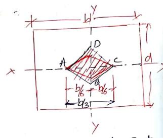
of omm is -ve, then stress will be tensile. But of omm is zero (& Positive) then there will be no tensile stress
