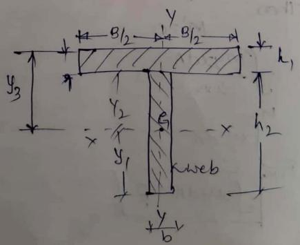
T section with flange Bxh, andlduse by has say by is the centroid the section on the axis yy, and XX & YX we the centroidal oxes Iny = Iney for flange + Ixy" for web for flange & vailies from - B/9 to + B/9 for web or varies from - b/g to + b/g Now, Ixy = S Sxy dxdy'+ (xy dydy Dx fydy + Ox fydy
