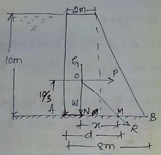
Thoust of earth on the vertical face of the wall is
