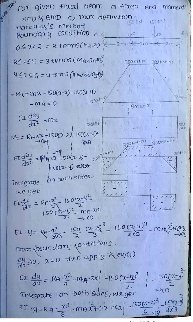
Apply Boundary conditions in equipos  $U \frac{dy}{dz} = 0, \quad x = 0$ [:- C=0 (2) y=0, x=0 Apply (18(2 in eq(1)) (3)  $\frac{dy}{dx} = 0, x = 6$  $EI.(0) = RH \frac{6^2}{2} - MH(6) + 0 - 150(6-2) \frac{1}{2} ISG(6-4)$ 0 = 18RA-6MA-1500 18RA-6MA = 1500- $EI(0) = RA(6)^{3} - mA(6)^{2} + 0 + 0 - \frac{150(6-2)^{3}}{6} - \frac{150(6-2)^{3}}{6}$ 0 = 36RA -36MA -1800 36RA - 38MA = 1800 - >(4) 1 : RA =150KN 1- MA = 200 KM-M RA+RB=150+150 RA+RB = 300 RB=300-150 F.RB = 150KN cmA=0
