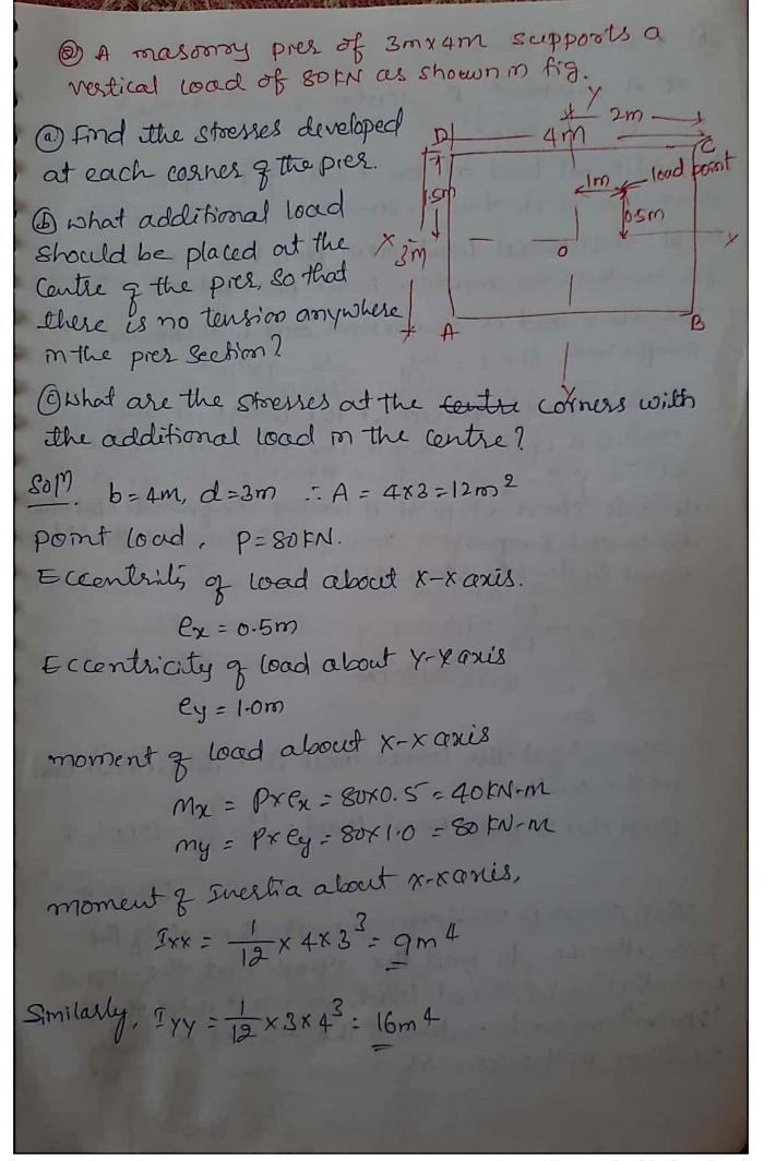
(a) Resultant Stresses at A = -10 kN/m2, B = 10 kN/m2, C = 23.33 kN/m2 D = 3.33 FN/m2
