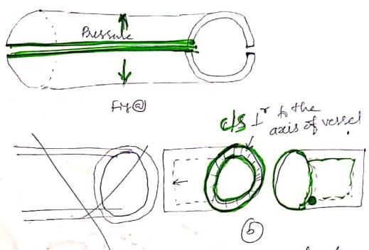
The forces, due to pressure of the fluid acting vertically upwards and downwoods on the thin cylinder tend to purst the cylinder &
