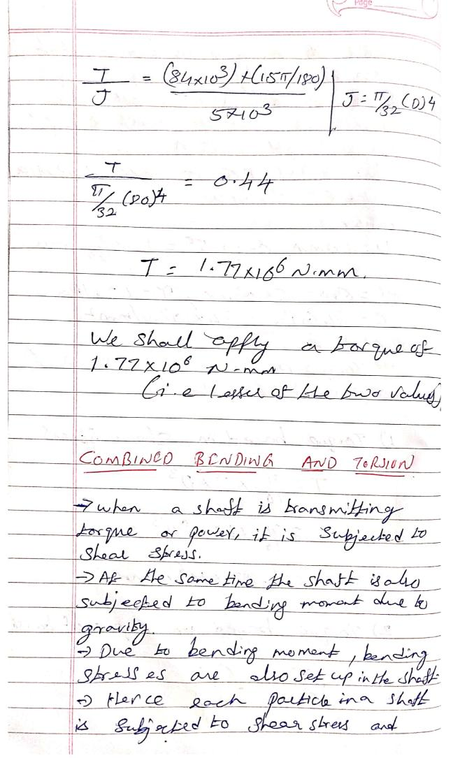
bending strais. bending of bending purpose it is recessary to Sind principle Stresses, Monimum sheal stress and strain energy. steal stress when a short is Subjected to bonding and torsion, are obtained as Shear Street T XR Bending Stress Mxy Mxy Bending stoess and Shear stress is maximum at a foint on the surface of the Short R= P/2 47 = D/2 Ob: 32M T= 16'T
