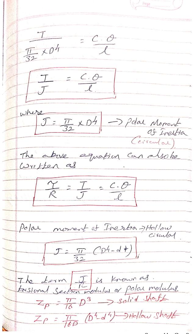
6. Calculate the maximum torque that a Short of Desmir tianater Can toansmit, if the maximum angle of twist is 10 inaleight of 1.5m. Take C= 70GPa Given: D-125mm, O-10=17 ind Length of Shoft: 1.5m = 1:5x103mm. C = 706pa = 70x103 N/mm2 Polar moment of Inertia of Bolid circula Shatt, J= T xD4 = II x 1254 = 24.0×10 min4 Relation for tarque transmitted by 7 (70×103) 11/180 T=19.5 KN.M
