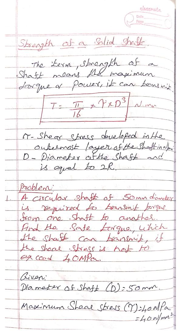
Safe Torque! T= 11 × Tx D3 = IT X40X503 0.982 KN.M A Solid Steel Short is to toansmit a torque of 10 km. m. Is He shooring stress is not to exceed 45 Mpa. Find the minimum diameter of the Shaff. aiven, Terque, T = 1012N.m: 10×16 N.mm 7= 45 MPa = 45 N/mm2 T= T × 7 × 10 3 10×1065 11 ×45×23 D3-1,132×106 = 1.04 ×102 = 104 mm
