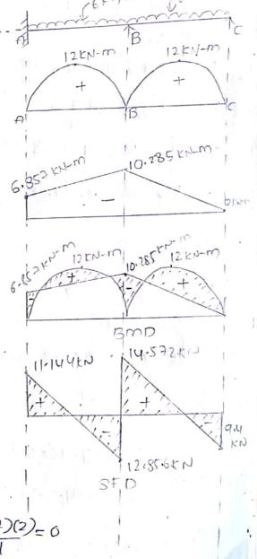
MALI+2MB(4+ 12)+ MC(12) + 60121+ 6011, MA(4) + 2MB(4+4) + 4(0)+ 6x32x2 + 6x32x2 - 6x32x2 16MB+4MA+192=0 -> (3) From eq (3) \$(2) 1: MA = -6.857 KN=m 1:MB=-10-285KN-M V=O
