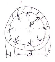
Fig shows a thin cylinderical vessel in which a fluid under thessure is stored.
