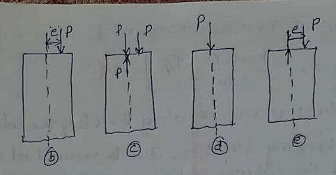
Resultant stress when a column of Rectangular section is subjected to an eccentri load
