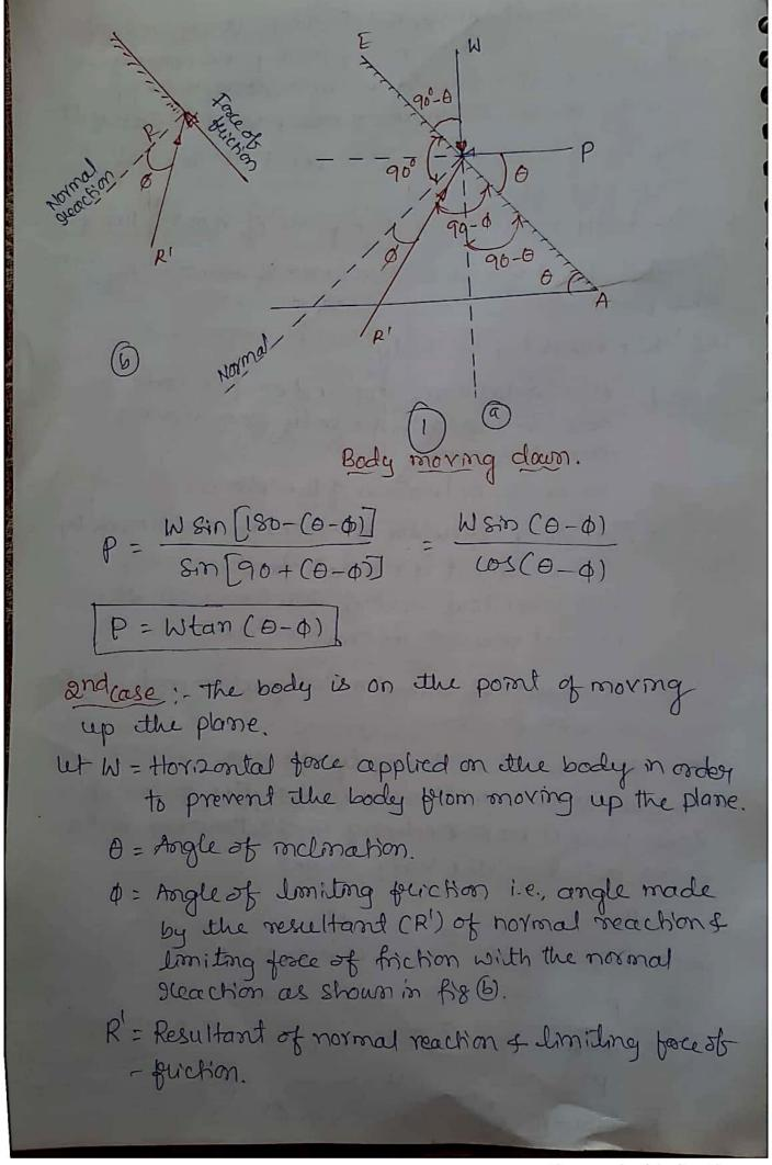
The fosce acting on the body are shown in fig 20. The body is in equilibrium under the action of three forces W. P+R Applying lamils theorem to the forces acting on the body, we get Some of angle dw W4R = Some of angle offw R4P Sin (90-0+90-0) = Sin (0+90+0) Sin (180-(0+0)) = Sin (90+(0+0))  $P = \frac{\text{Wsin} \left[180 - (\theta + \phi)\right]}{\text{Sin} \left[90 + (\Theta + \phi)\right]}$ P = Wtan (0+0)
