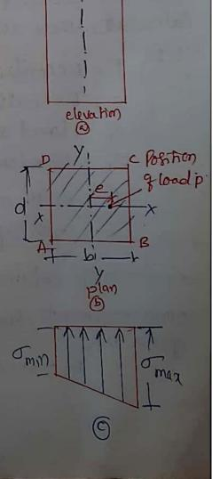
The resultant stress at any point will be the algebraic sum of direct stress & bending stress
