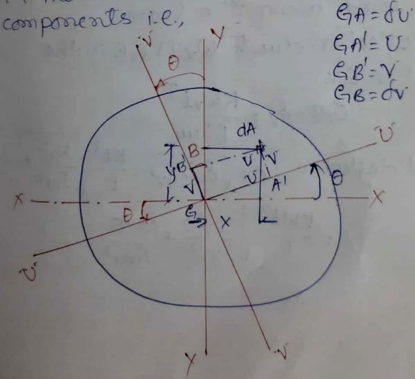
Wu = Wsmo (along UG dreckon) Wy=Wcoso (along VG direction) Say deflection due to kly is GA m the direction GV. 1. e. GA= Oce - K. We. L3 where K is a constant depending upon the end conditions of the bearns possion of the bearns Deflection due to Why is & B in the dreckon GV. GB = 8v = KINVL3 EJUY Motal deflection, &= | Suttov2 = E | Ivv2 lui 6 = KW13 | Sm20 + cos20 Tyv2 + Tuc2
