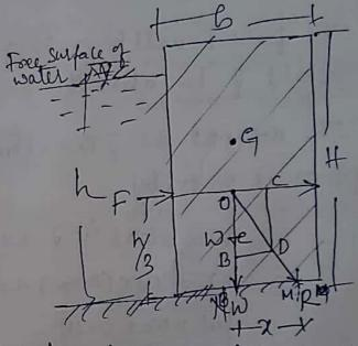
Fig shows rectangular dam having water on one
