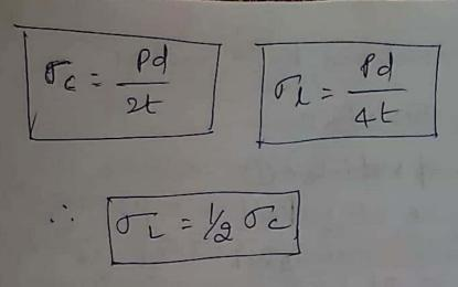
this also means that crocumferential stocks (oc) is two times the longitudinal stocks (oc) Honce in the material of the certification the reaction of the certification than the crocumferential stocks.
