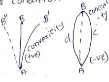
? A moment which will tend to bend the column with its concavity towards its initial centre line. Taking as "-ve".
