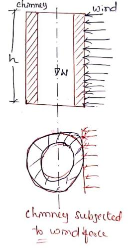
The wind force (F) acting in the horizontal direction on the swiface of chimney is given by.
